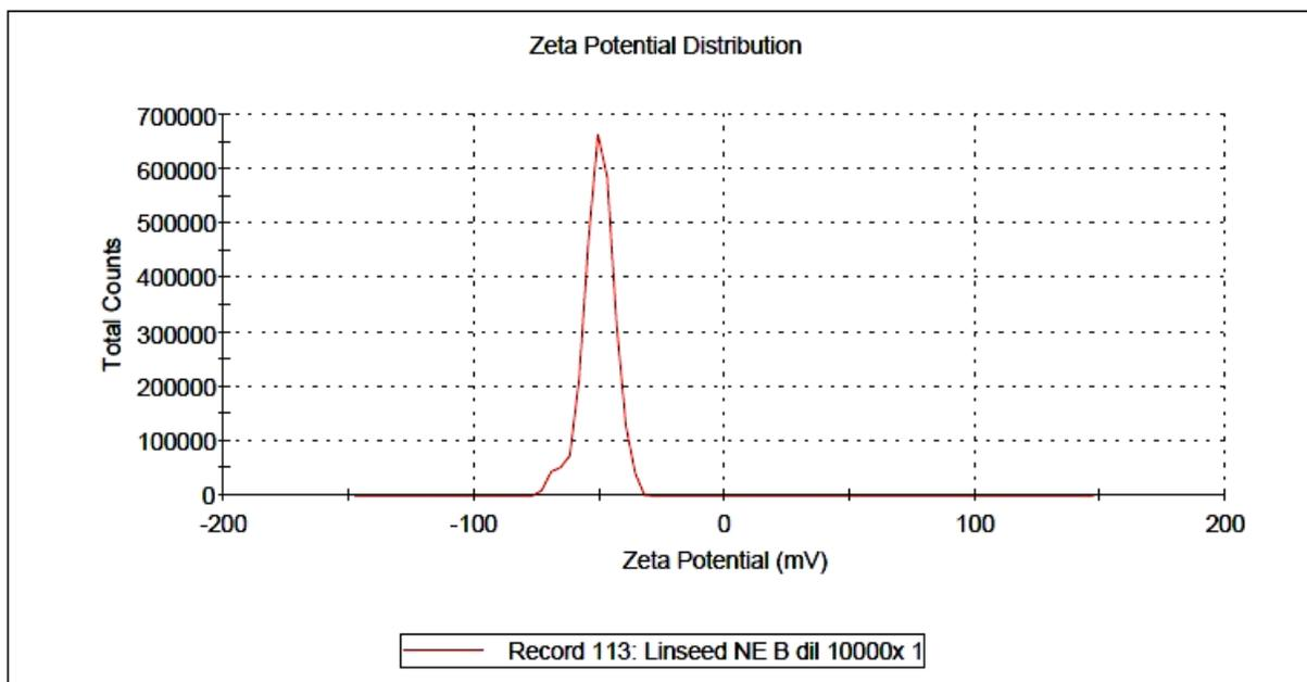
Figure 3: Zeta potential analysis of losartan loaded nanoemulsion (F5).
