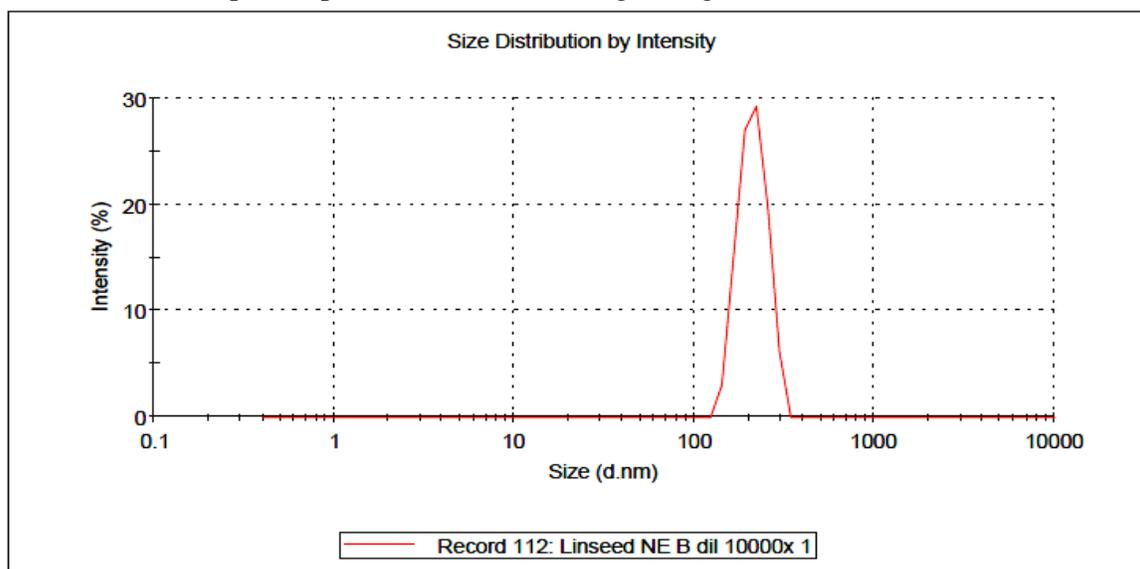
Figure 2: Droplet size distribution of losartan loaded nanoemulsion.
