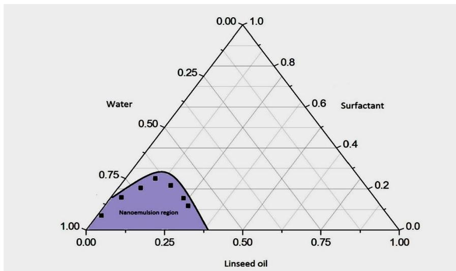
Figure 1: Pseudo-ternary phase diagram of linseed oil, surfactant (Span80 and Tween 80 in ratio of 1:2) and aqueous phase. The darkened region signifies the nanoemulsion zone.
